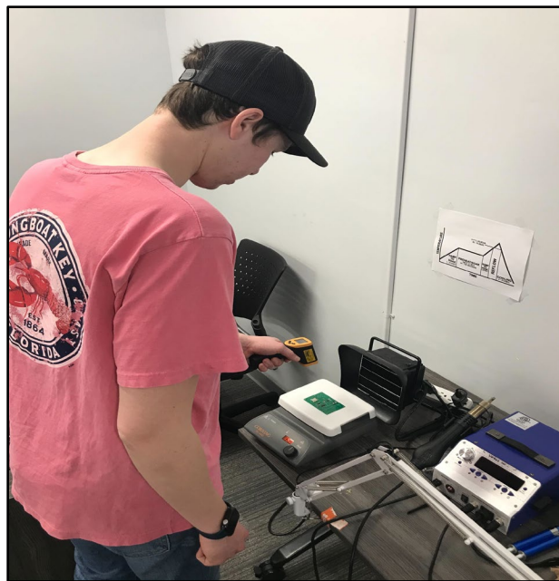
Fig. 2.35. Performing Reflow Process with Heated Bed
